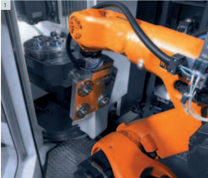
I1+2I Automatic pallet handling and a pallet magazine with 20 pockets
