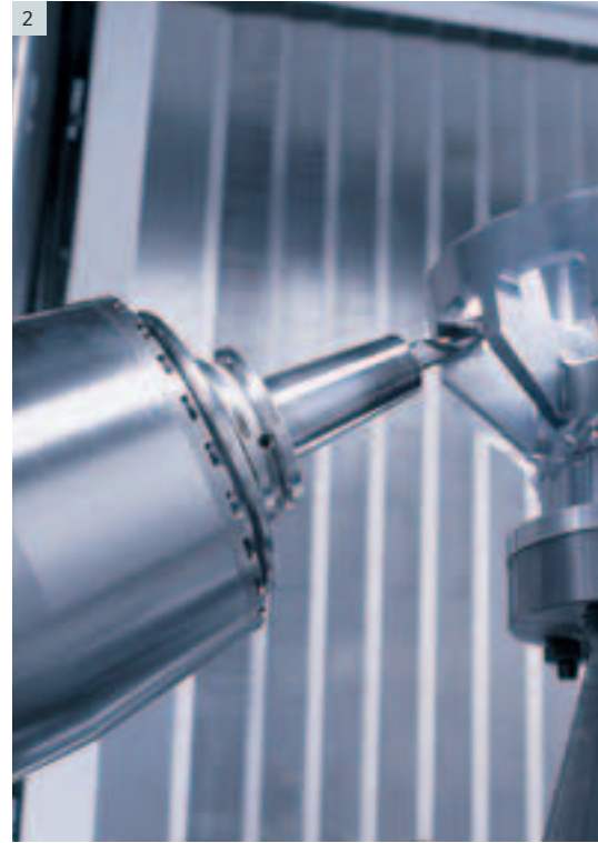
I1| Large work area with the integrated NC rotary table and the NC-controlled milling head (optional, standard for the DMU 40)
