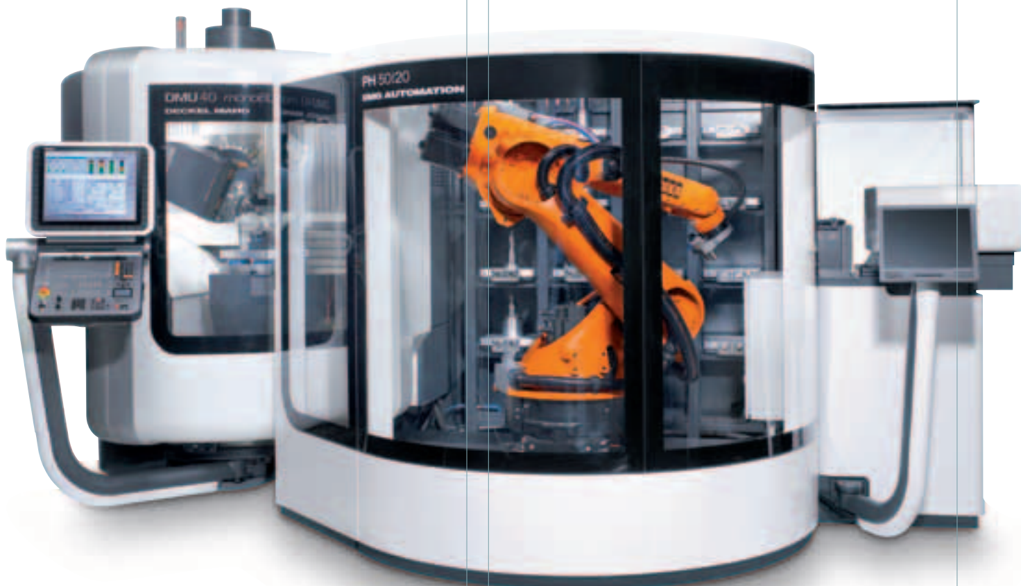
Automation solutions for the monoBLOCK® series: e.g. DMU 40 monoBLOCK® with an automatic loading and unloading system with a 6-axis robot, pallet-hand- ling system with a pallet weight of 50 kg and 20 pockets.
